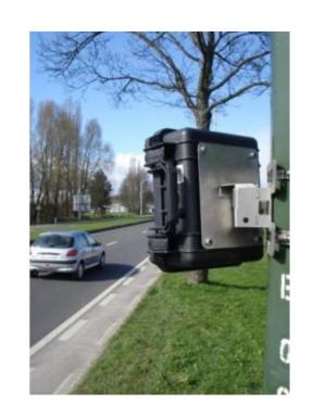
Typical radar installation
